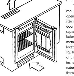
The minimum total area required for ventilation openings depends on the size of the fridge. All **single** door Nova Kools require 60 square inches of total ventilation area. It is recommended that the vents are located at the bottom (30 square inches) and the top of the fridge (30 square inches); this supports the natural convection of heat from cold (bottom) to warm (top).
