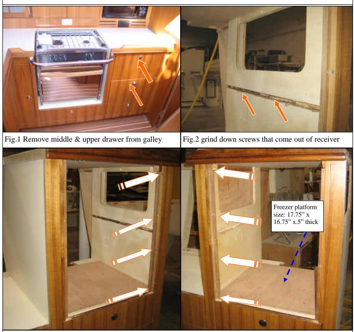
Fig.3 Mount & install wood part face trims on freezer compartment face panel, secure mounting screws as arrow indicated directions. Install freezer platform as shown illustration above.
